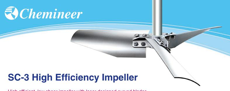
High efficient, low shear impeller with laser designed curved blades providing high strength and low weight which is ideal for long overhung shaft applications
