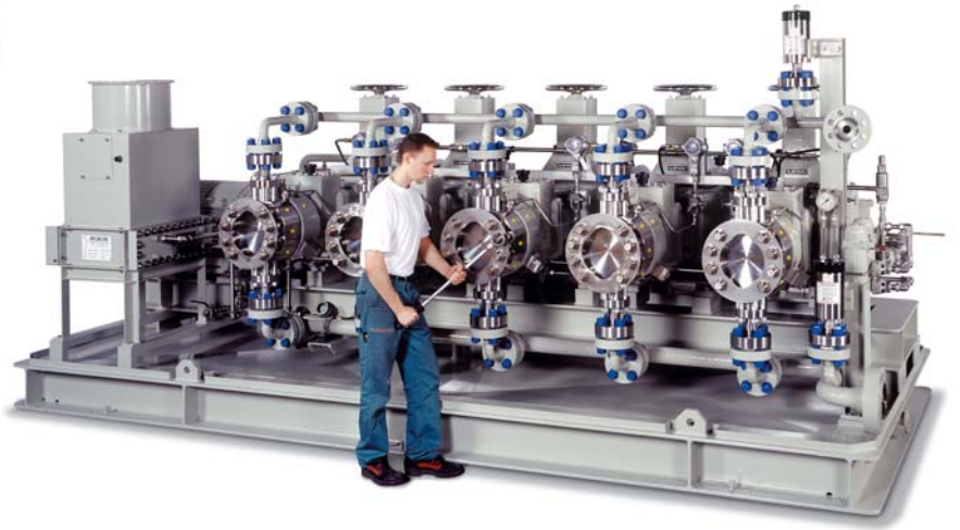
Example upstream oil & gas industry: methanol injection, 8,8 m 3 /h at 345 bar, M500 for hydrate-formating protection
